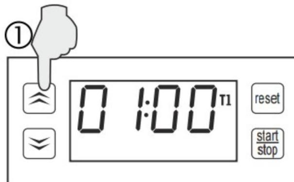
Press the UP button for 3 seconds. CLOCK symbol and T1 light up and the second display starts to flash.
