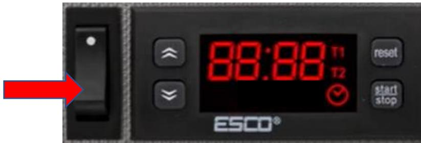
Press the main switch to switch on the Air Mentor.
